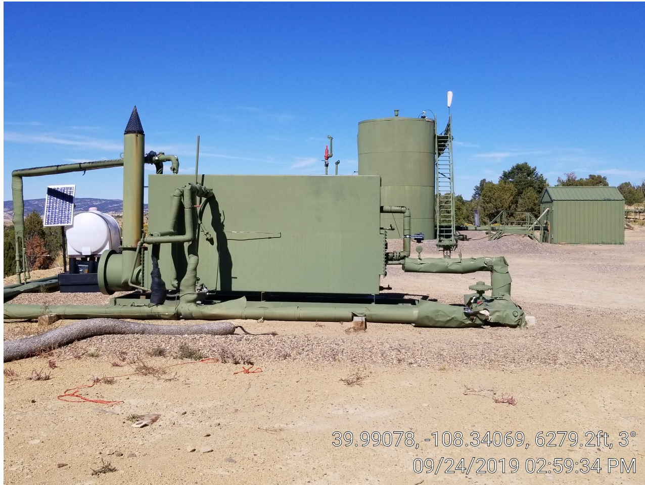
Photo 2. Separator, tanks, and equipment building.
