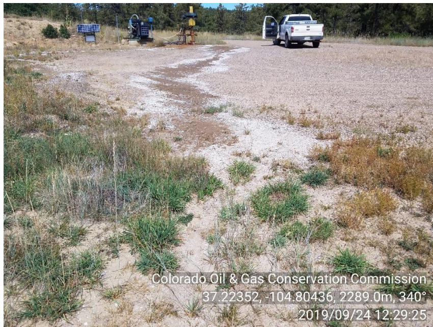
PHOTO 3: APPEARS THAT PACKING WAS LEAKING ON WELLHEAD (NOT THERE IS NO LEAK AT TIME OF INSPECTION). IMPACTED AREA EXTENDS FROM WELLHEAD TO SOUTHWEST APP. 123'. Control and contain spills/releases and clean up per Rule 906.a. Contact COGCC EPS staff. CA DATE 9-25-19.
