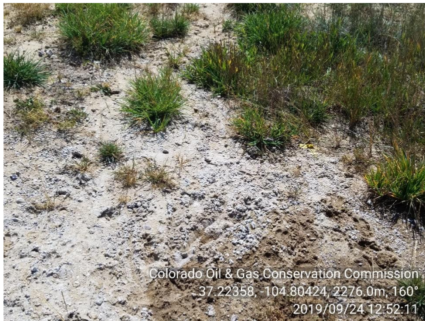
PHOTO 5: PHOTO SHOWING THAT THERE HAS BEEN OTHER EVENTS AS YOU CAN SEE THE WHITE CHALKY STAINING BEYOND THE CURRENT WET SOIL. WHITE CHALKY STAINING EXTENDS PAST CURRENT WET SOIL APP. 18'.
