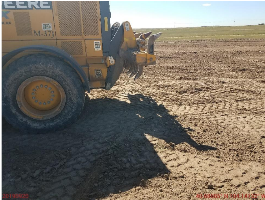
Photo 19: Photo shows ripper teeth used to conduct compaction alleviation. Photo shows used to conduct compaction alleviation are not sufficient in size to rip to a minimum depth of eighteen (18) inches in accordance with 1003.c.
