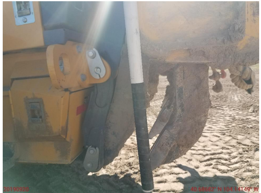
Photo 20: Continued from photo 19. Photo shows teeth used to conduct compaction alleviation was approximately 1 foot in length.
