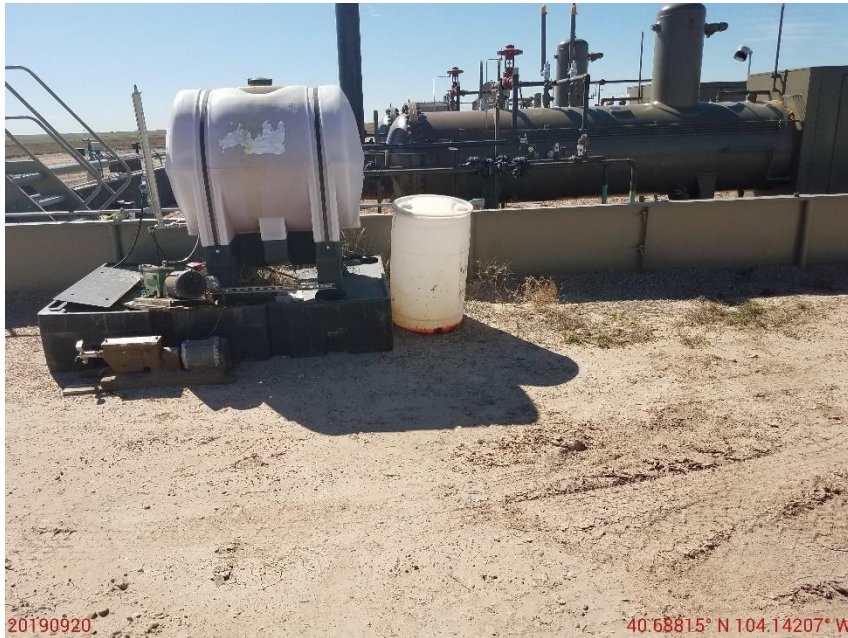
Photo 7: Photo taken from the north end of the location. Photo shows container previously identified has not been placed in secondary containment. Photo also shows required labeling identifying contents remains missing.
