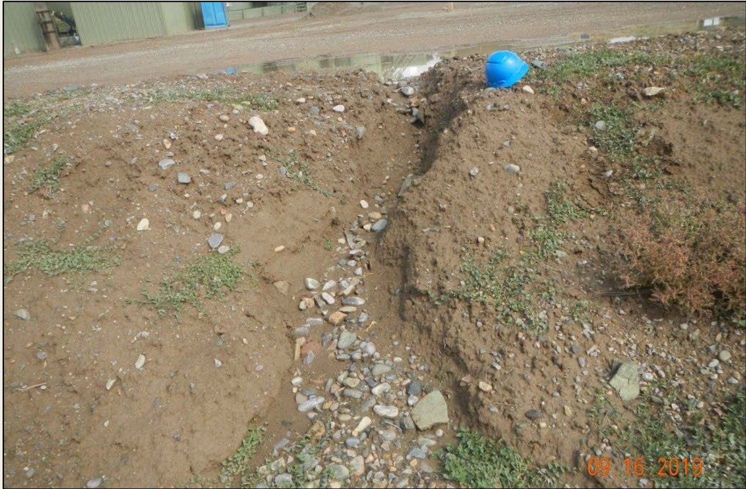
Photo 3. View of erosional channel approximately 2 feet wide and deep within the southern project area.
