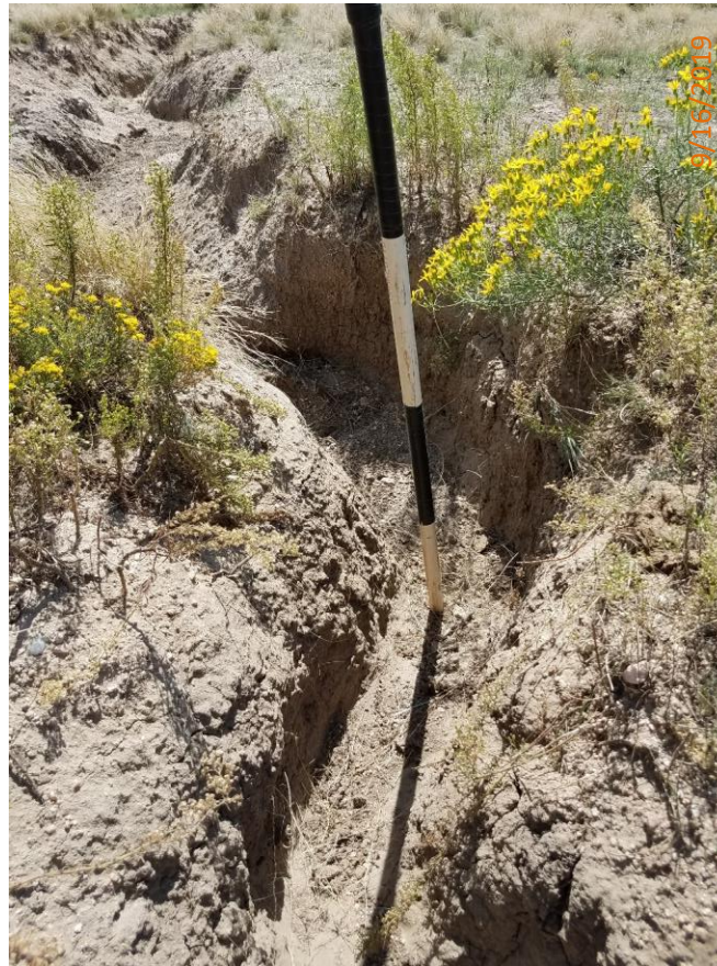
Photo 15: Photo taken from the gully forming to the south of the location. Robel pole for reference. Each white/black marking on pole represent \frac{1}{4} meter (0.8 feet). There are areas of the gully that are 1.5 to 2 feet in depth.
