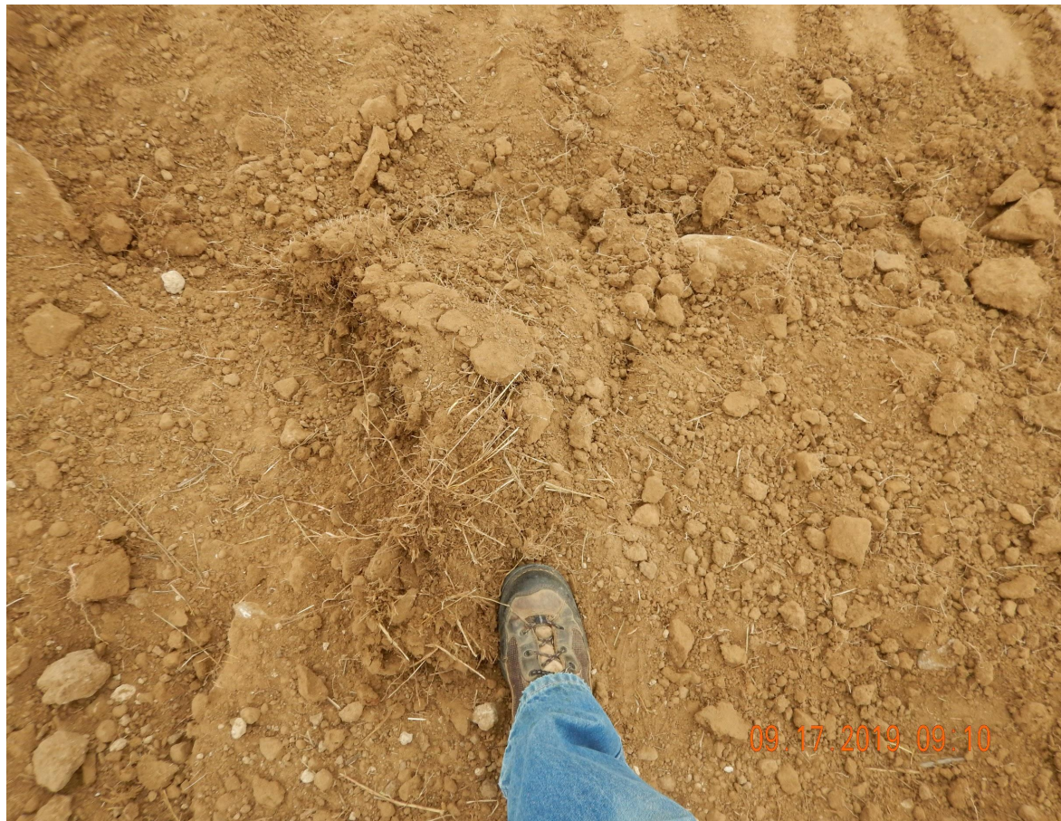
Photo 11. Close up photo taken from the northwestern well pad location. Photo illustrates characteristics (root growth) of the topsoil horizon as confirmation of topsoil being used as fill material.
