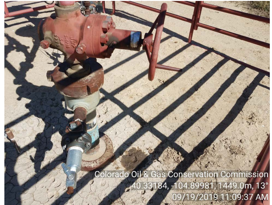
Master valve and stained soil on Gold 11-9DU
