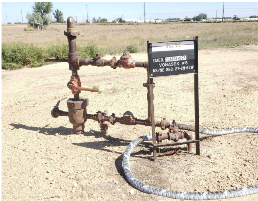
Photo #1 WH with PU removed.
