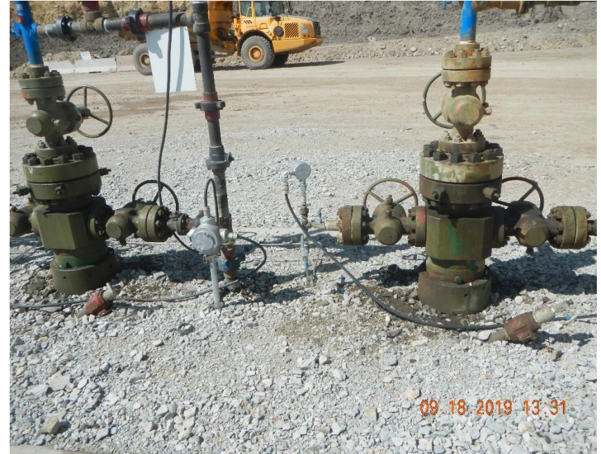
Stained ground surfaces at and around wells.
