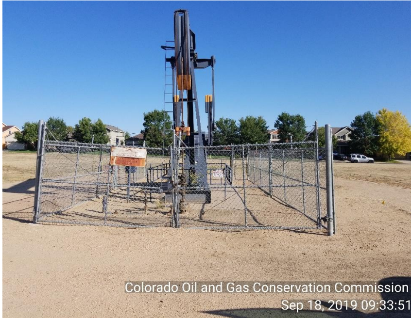
Photo 1 PU and WH. KPK in stalled a used old sign, but sign is legible.
