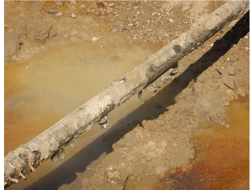
Close up view of flowline at the point of failure (coating is hanging down). A clamp was observed where a historical repair was completed.
