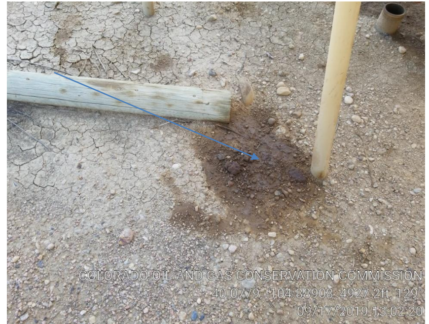
Pic 8 stained soil/possible leak on bottom of tank
