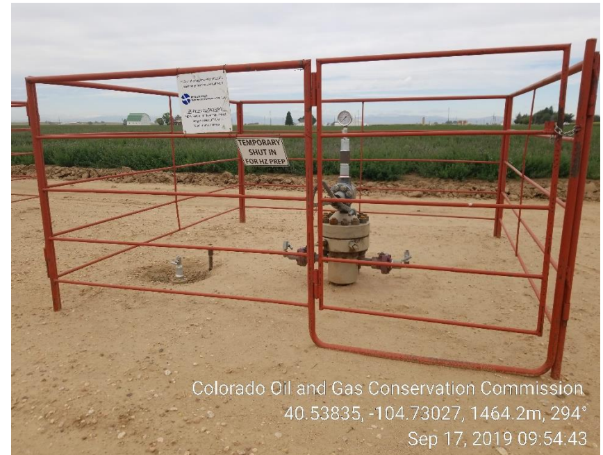
Photo 2: (TA) Wellhead
