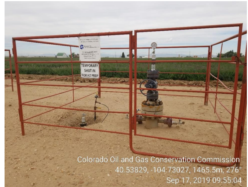
Photo 2: (TA) Wellhead
