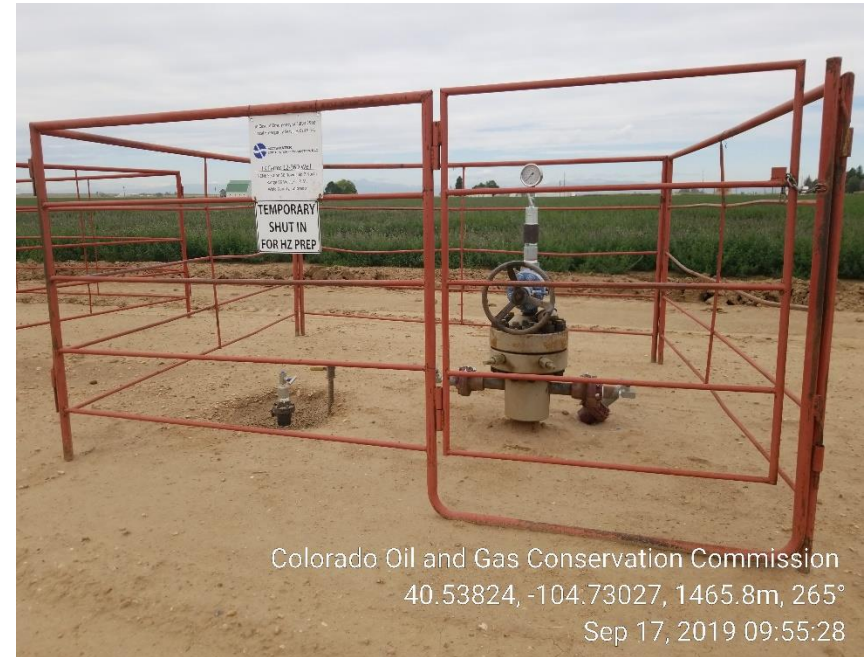
Photo 2: (TA) Wellhead
