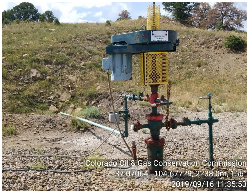
PHOTO 1: WELLHEAD/ UNUSED RISER. REMOVE UNUSED RISER, COMPLY WITH NTO. CA DATE 10-16-19
