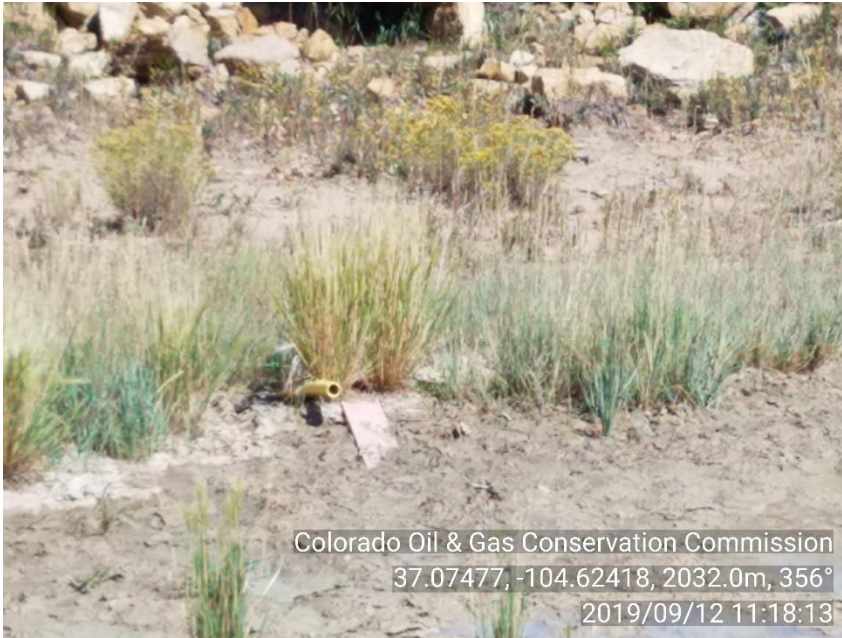
PHOTO 5: GUY LINE ANCHOR MARKER IS DOWN. Install proper guy line markers per Rule 1003.a
