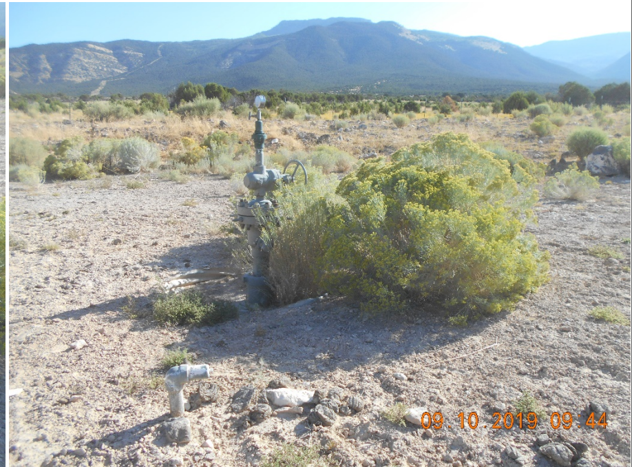
Wellhead looking N. Temporarily abandoned Unused 2" riser with plug in foreground.
