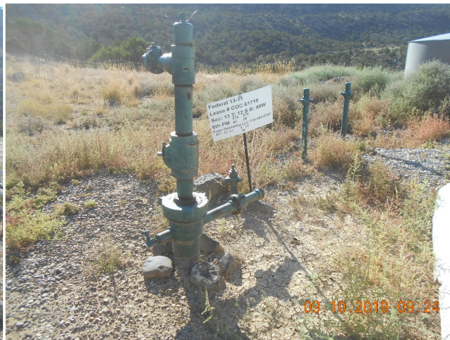
Wellhead with sign. Temporarily abandoned. 3 x 2" unused risers with plugs.
