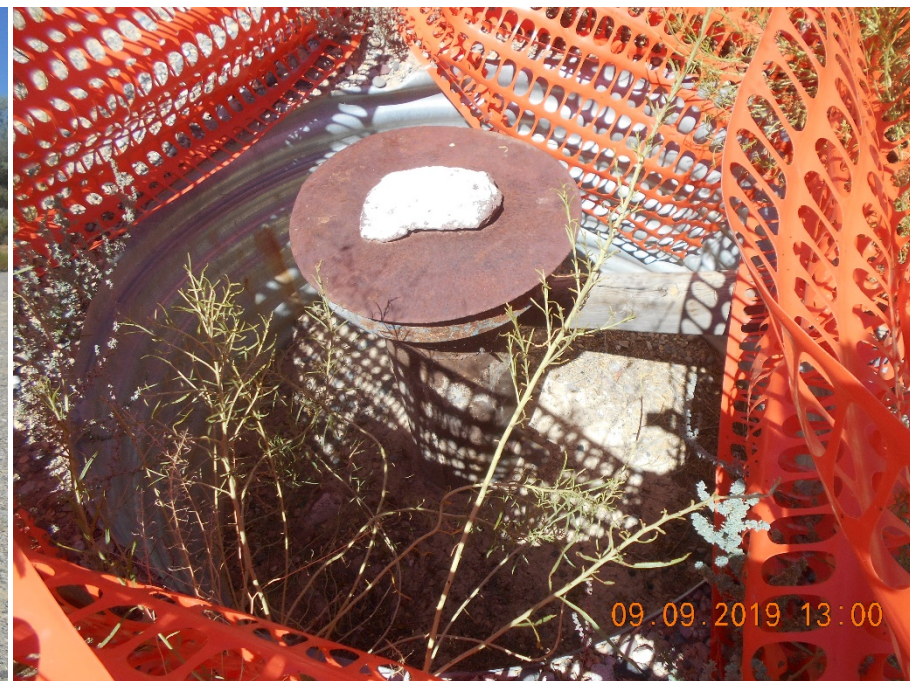
Surface casing with cover plate in corrugated cellar.
