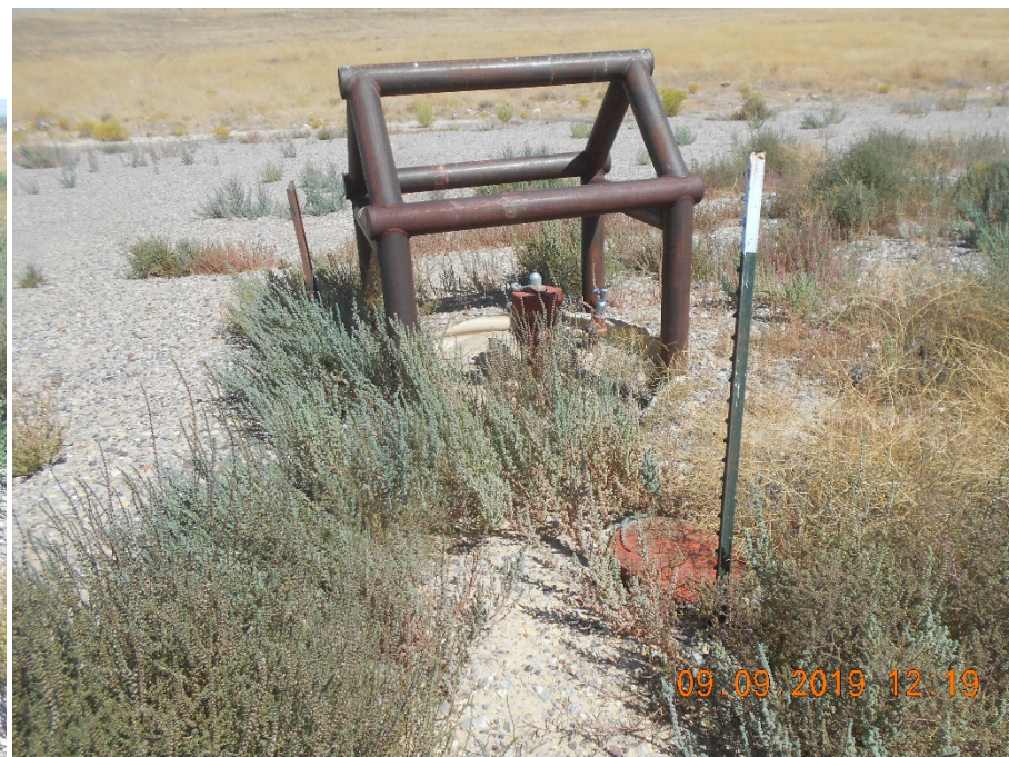
API # 05-077-09459 Kelly #23-2-B Wellhead with sign and pipe barricade looking N. Rat hole with cover next to T-post in foreground.
