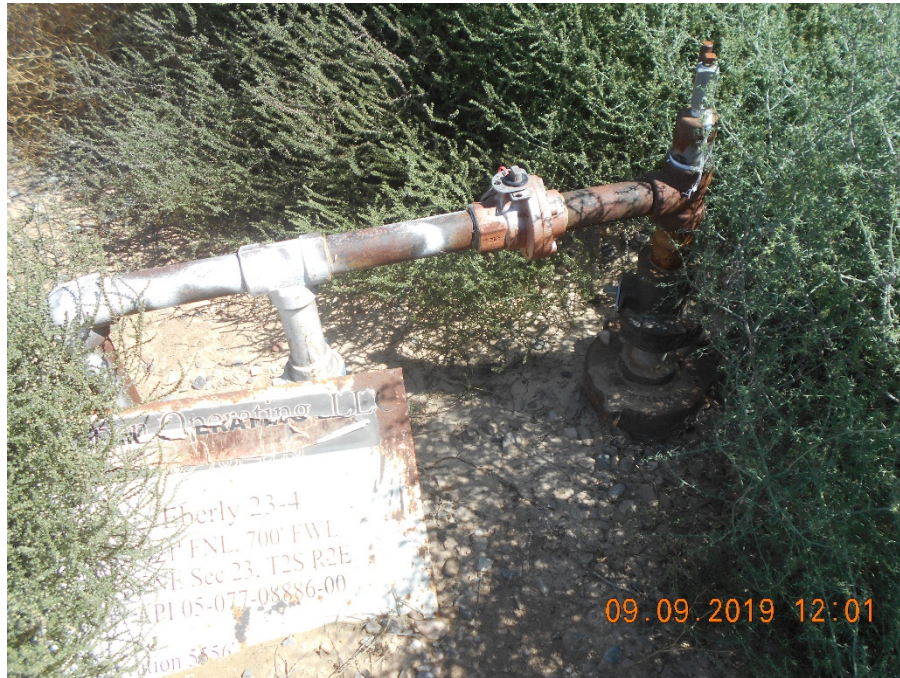
API #05-077-08886 Wellhead with sign. Temporarily abandoned. Overgrown with weeds.
