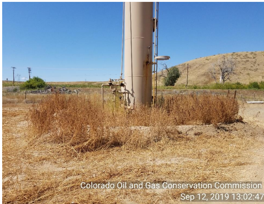
Photo 9 vertical separator. WEEDS in and around containment
