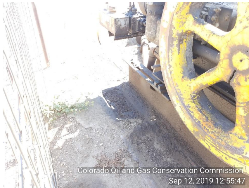
Photo 5 stained soil around PU motor
