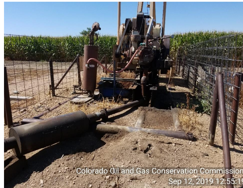
Photo 4 Stained soil around PU motor
