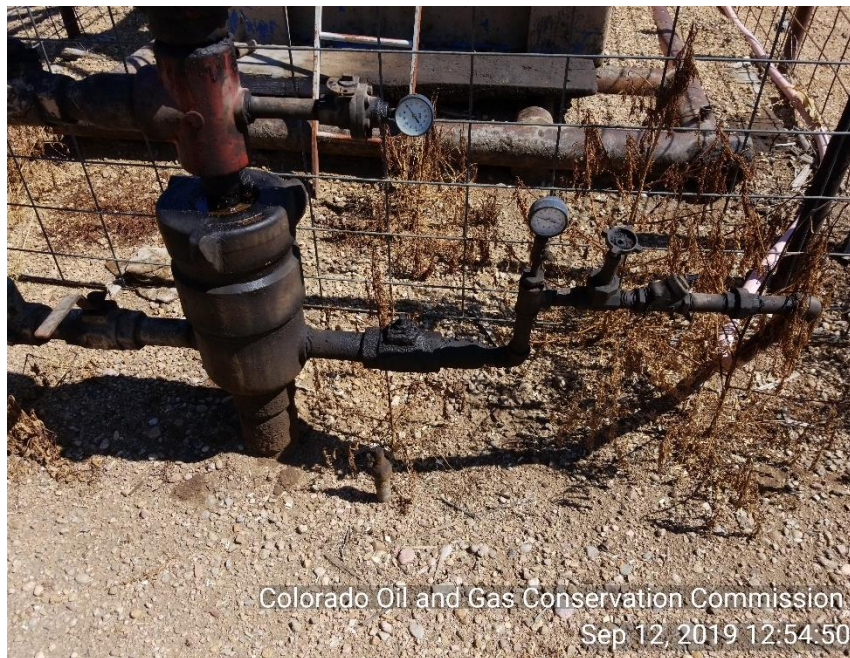
Photo 3 stained soil around WH
