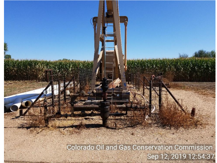
Photo 2 WH Stained soil around WH. Debris: dead weed around well head.
