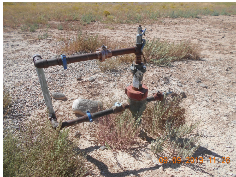
Wellhead. Locked out / tagged out. Weeds
