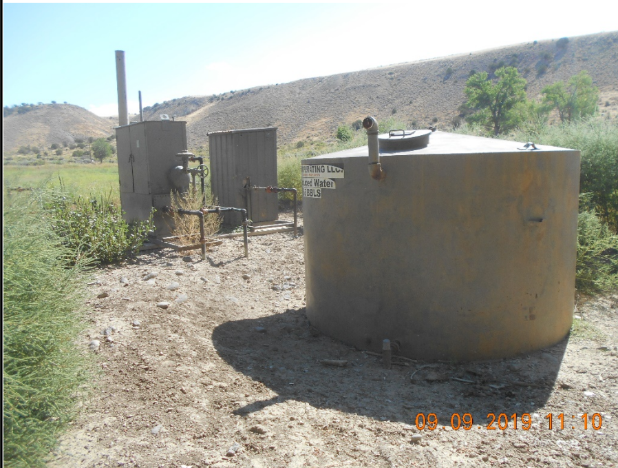
Tank, Meter housing and Separator looking E. Disconnected riser with plug at base of tank Berms inadequate. Weeds
