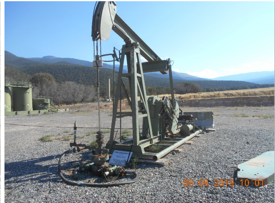
API # 05-077-09470 Mansur 33-1-L wellhead with sign and pump jack. Temporarily Abandoned
