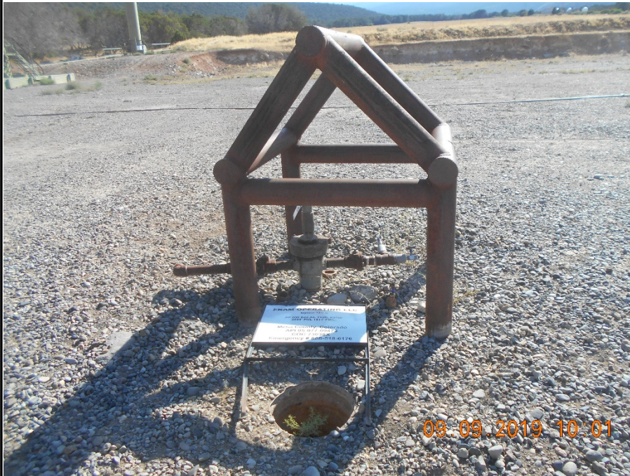
API # 05-077-09473 Mansur 33-1G wellhead with sign. Temporarily Abandoned.
