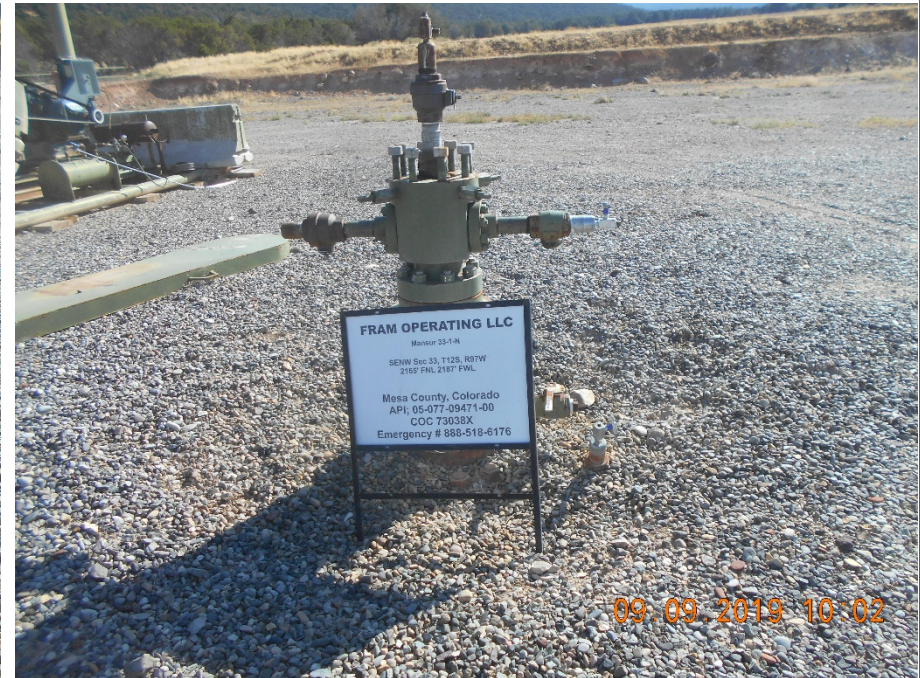
API # 05-077-09471 Mansur 33-1-N wellhead with sign. Temporarily Abandoned
