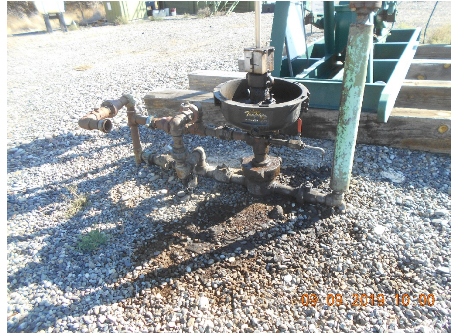
API # 05-077-09475 Mansur 33-1K wellhead with stained soil.
