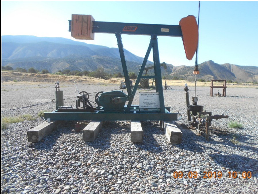
API # 05-077-09475 Mansur 33-1K wellhead with sign and pump jack. Temporarily abandoned
