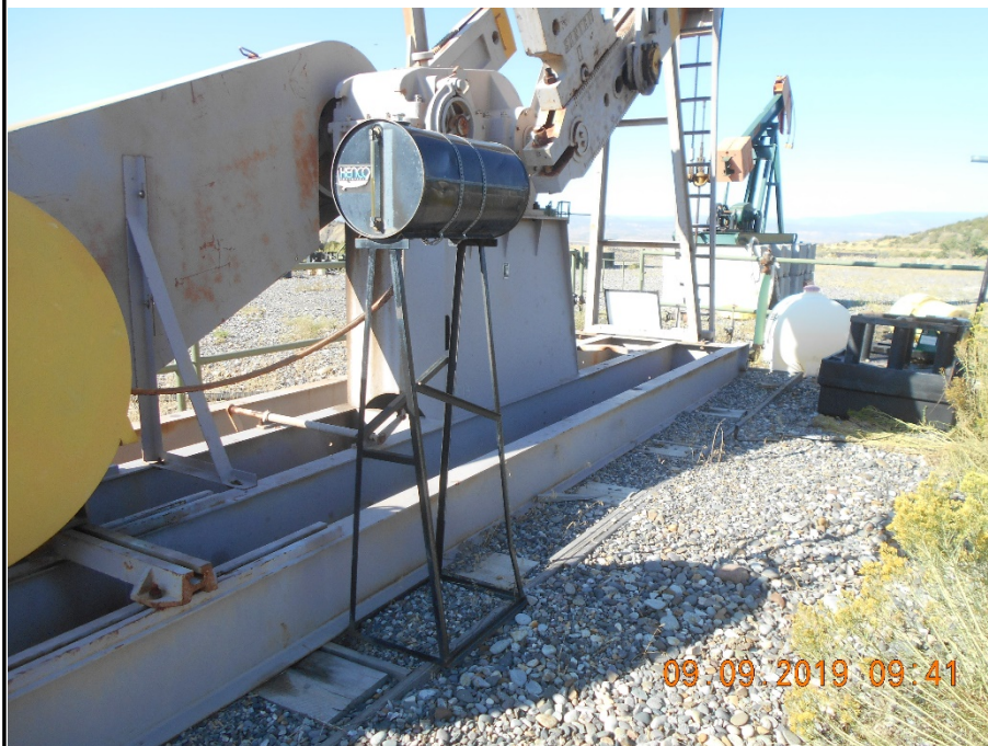
Lube oil tank for pump jack with no secondary containment.
