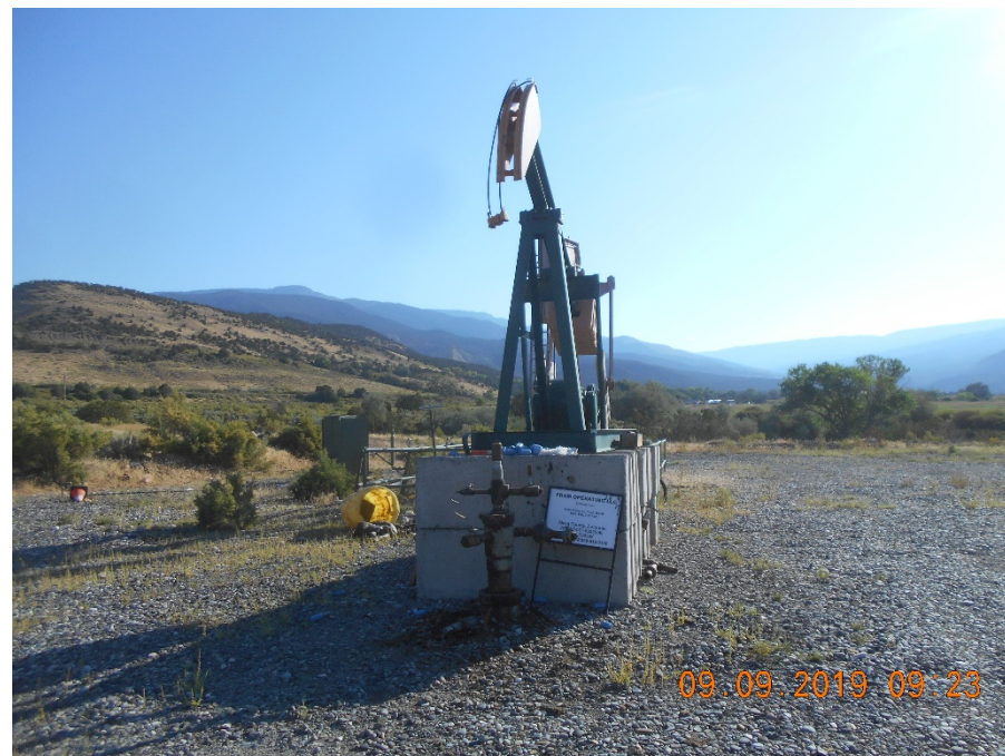
05-077-09325 Seminoe 32-2-I. Looking E Well Temporarily abandoned. Pump Jack disconnected Stained soil around wellhead. Vandalized spill response kit in background
