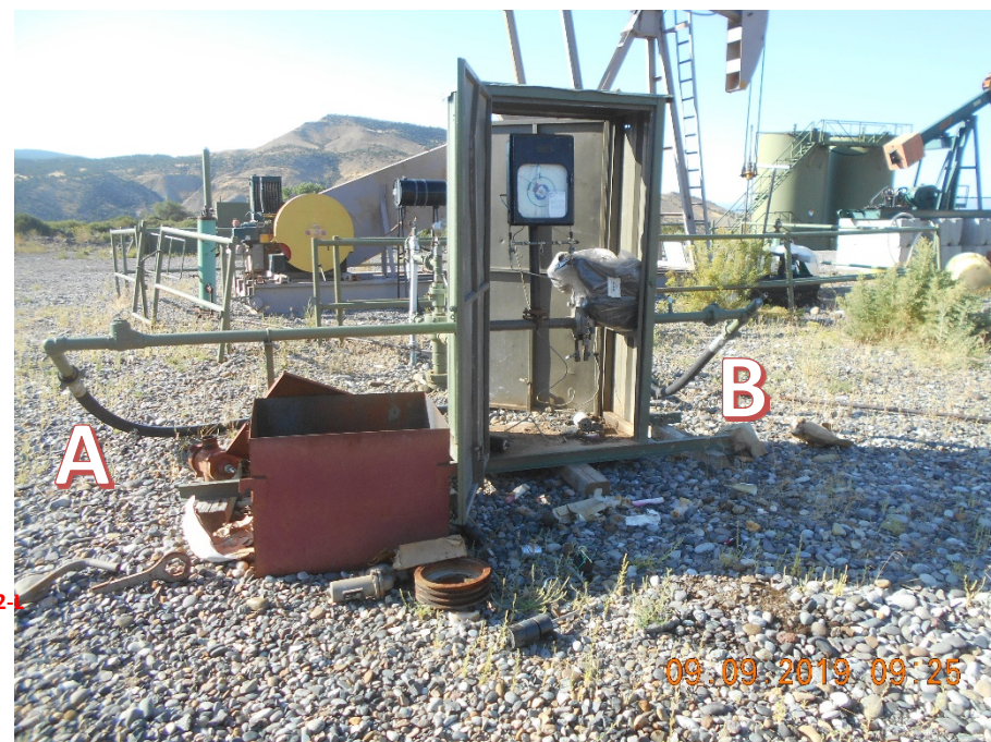
Meter housing with sides open. Looking S. 2" hose connected to wellhead flowing to meter. (A) 2" hose from meter to production riser at wellhead. (B) Parts, pipe and fittings scattered around .
