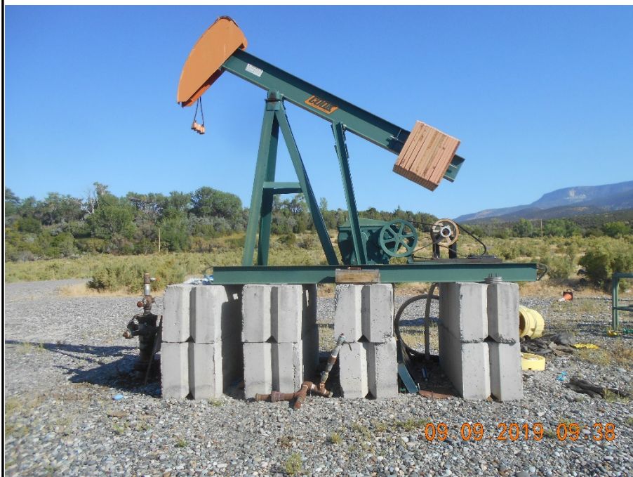
05-077-09325 Seminoe 32-2-I. Looking N Well Temporarily abandoned. Pump Jack disconnected. Pump Jack motor removed. Vandalized spill response kit in background.
