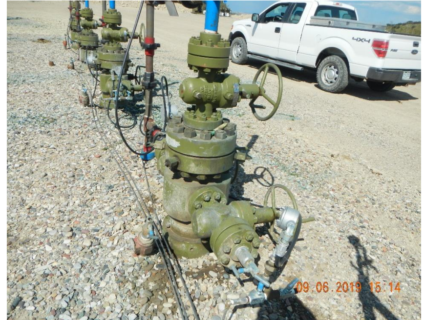
Stain soil around well heads.
