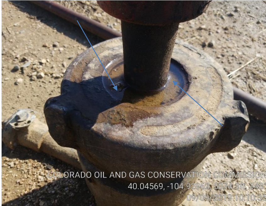
Pic 3 venting wellhead
