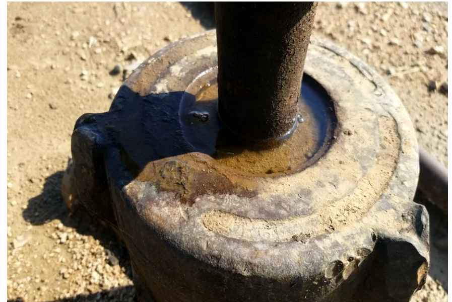
Video of leaking wellhead
