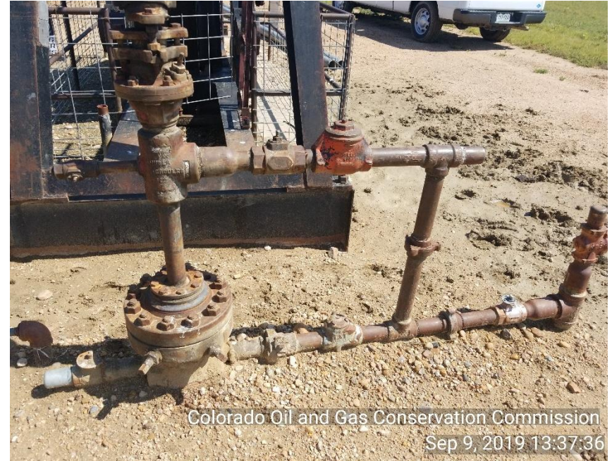
Photo 2 at time of inspection flow lines off well head are closed.
