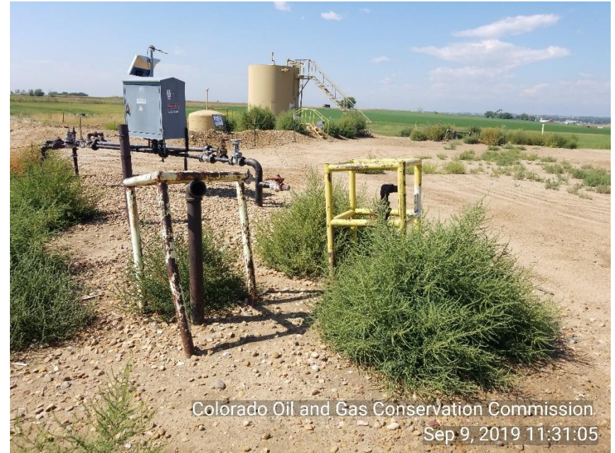
Photo 4 Unused equipment: unmarked not LOTO risers. WEEDS.
