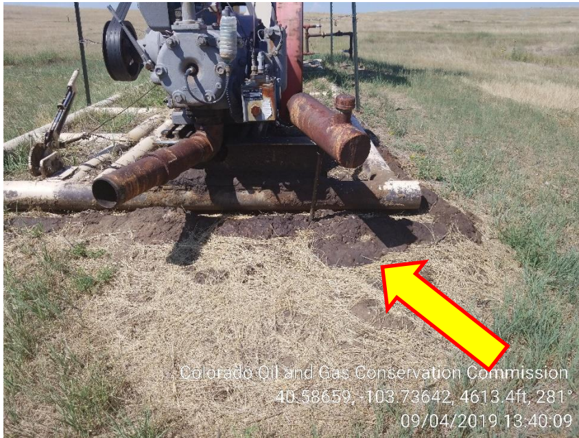
Photo 3 – Stained Soil at Gas Engine
