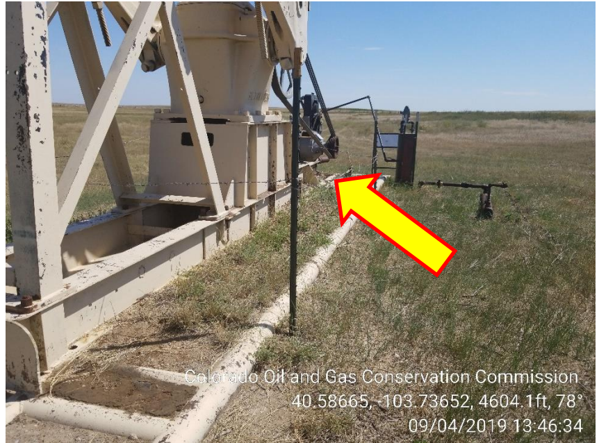
Photo 6 - Protective guard around Pumping Unit crank arms has been installed.
