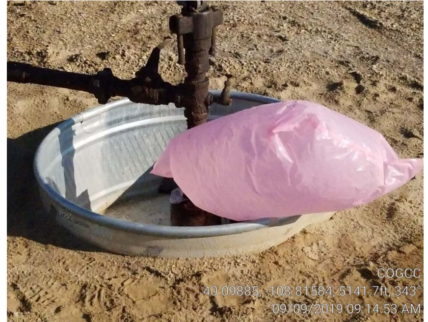
Photo 15. Gas venting into 3 cubic ft bag - Stragner 2.
