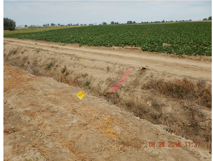
View release point marked at irrigation ditch; off location flowline marked with pin flags. View NW toward wellhead.
