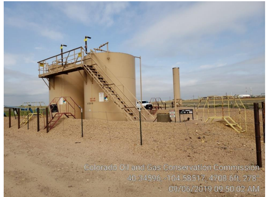
Photo #2 Tank Battery
