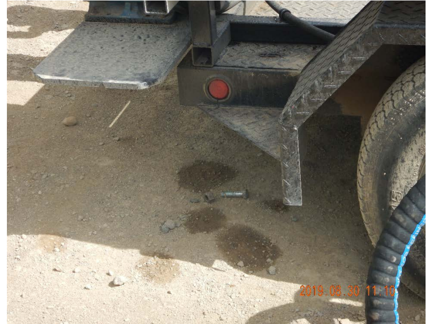
Photo #14 – Localized accumulations of oil-stained soil beneath trailer pump in previous photo.
