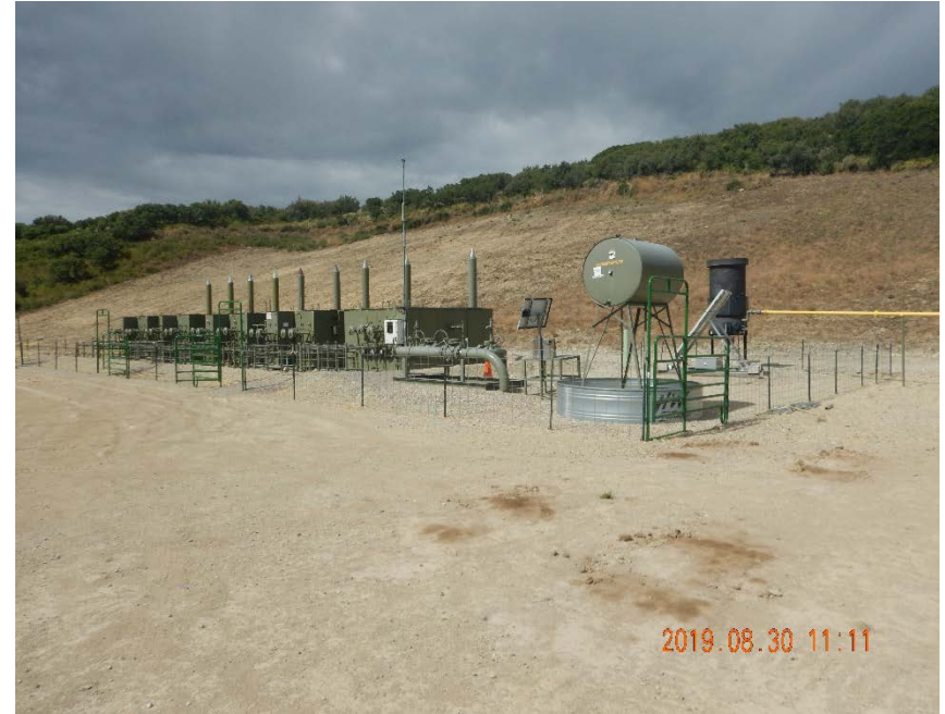
Photo #16 – View of heated horizontal separators, ECD, and day tank from northeast. Note localized accumulations of oil-stained soil NE of fenced separator area.
