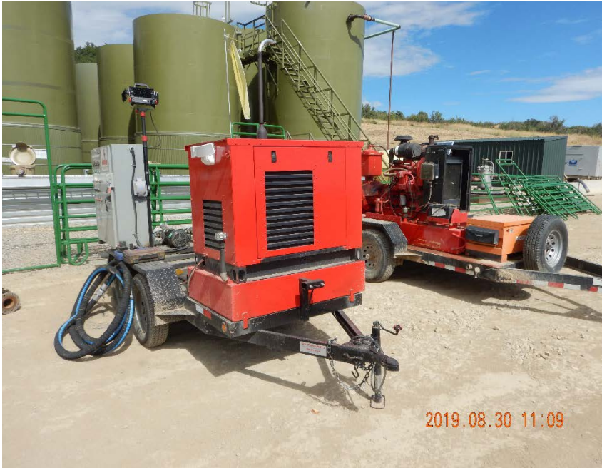
Photo #13 – Trailer pumps located east of tank battery lack secondary containment.
