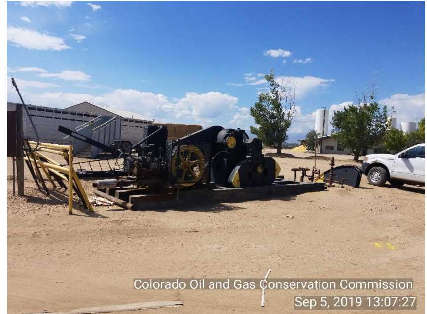
Photo 4 Unused equipment: PU and assoc. parts
