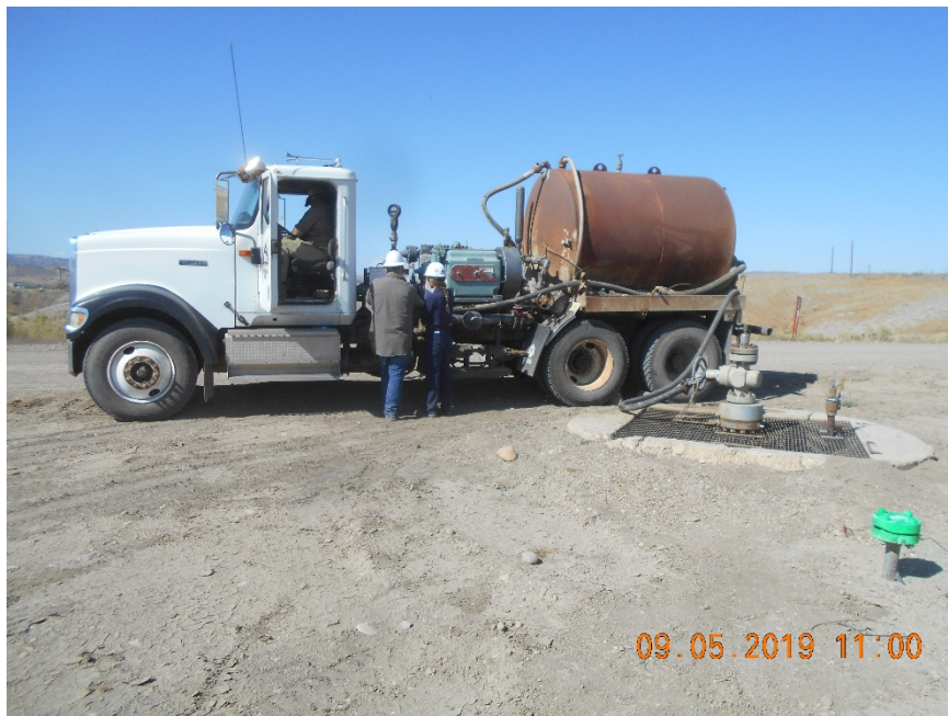
Injection wellhead with sign. Preparing for MIT.
