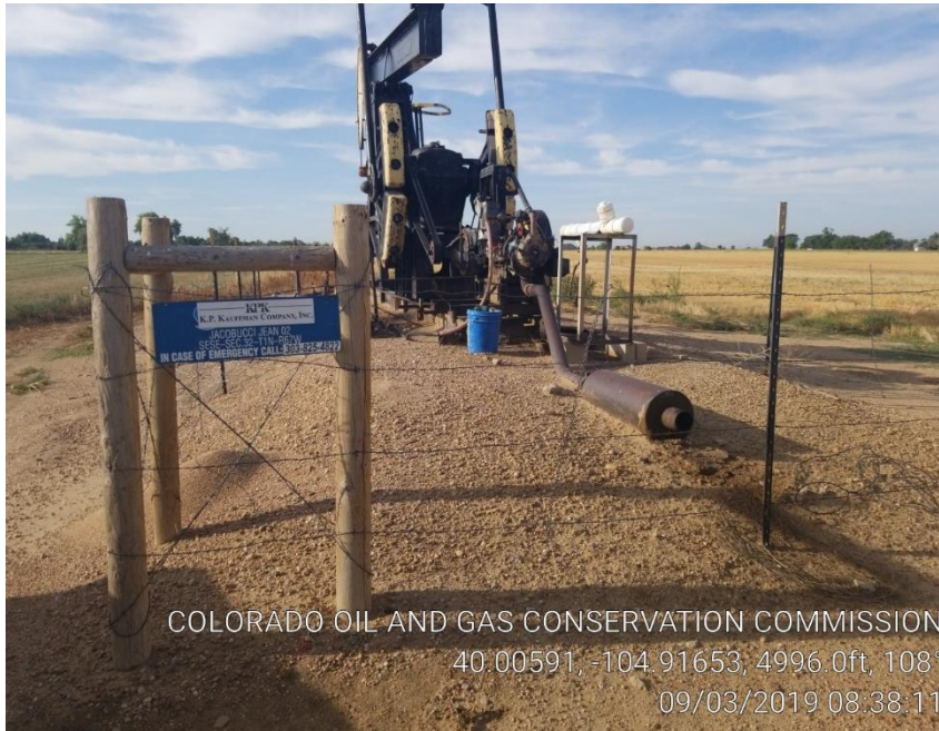
Pic 3 wrong operator and number, stained soil near muffler, blue bucket not in containment/trash
