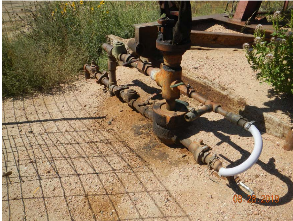
Photo # 2 - 05-087-07047 – Oil stained soil at wellhead
