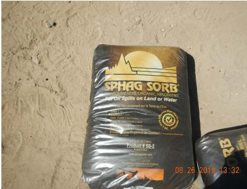
Photo #21 Sphag Sorb, peat fiber material that was applied to water surface.
