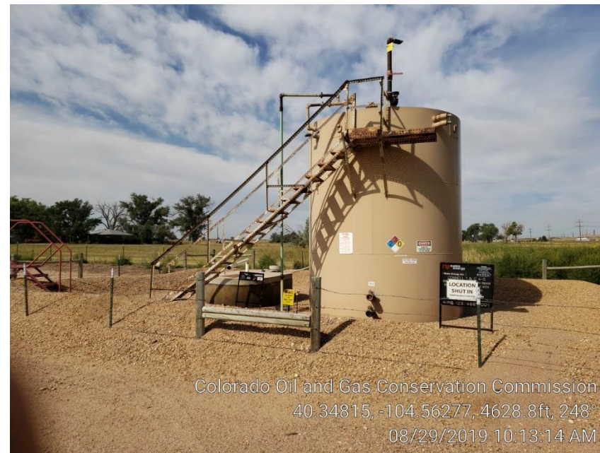
Photo #4 Tank Battery
