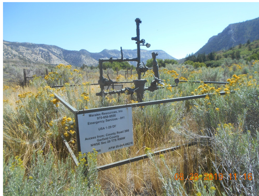
Wellhead with fence and sign - Temporarily Abandoned.
