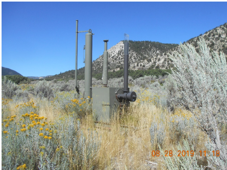
Separator overgrown with vegetation.
