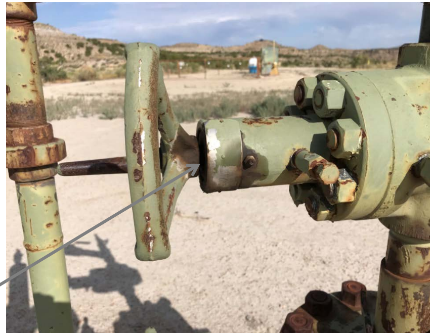
Photo 3. Gas leak.
