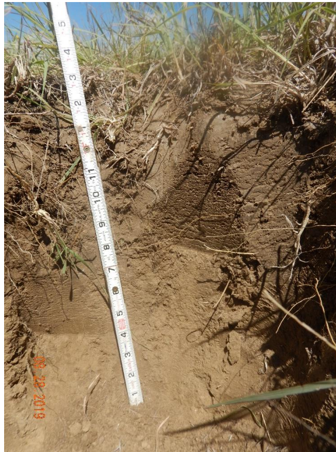
Photo 13: Photo of test pit from the reference area. Photo shows soils observed on the location are not reflective of soils on the adjacent reference area. Soils in the reference did not contain a chemical smell detected in the soils on the location.
