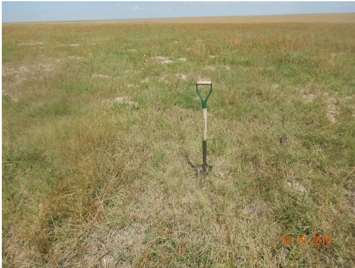
Photo 12: Photo taken from the adjacent reference areas. Photo shows reclamation specialist was able to easily penetrate the top 12-15 inches of soil. Compaction concerns appear evident on location. Reclamation specialist dug a test pit within the reference to compare soils observed on location.
