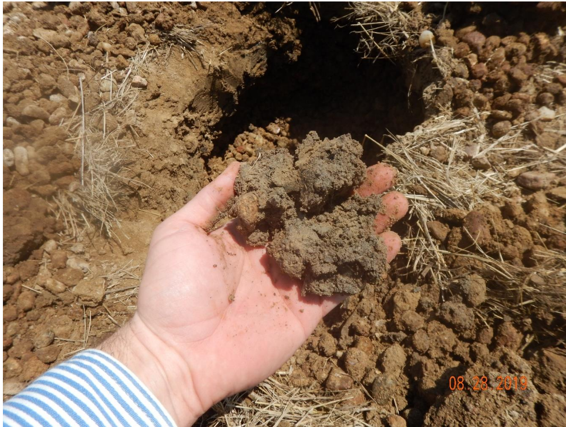
Photo 11: Photo shows additional soils excavated from the test pit. Similar to the gravel, soils also had a liquid sheen and a chemical smell.
