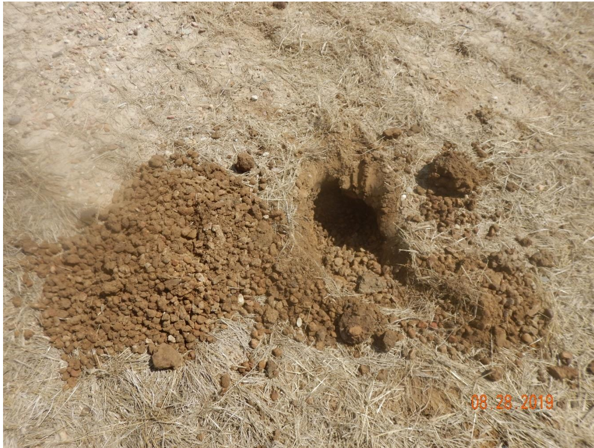
Photo 7: Photo taken from the location. Reclamation specialist conducted a test pit for both compaction and soil concerns. Reclamation specialist observed large quantities of gravel a few inches subsurface.
