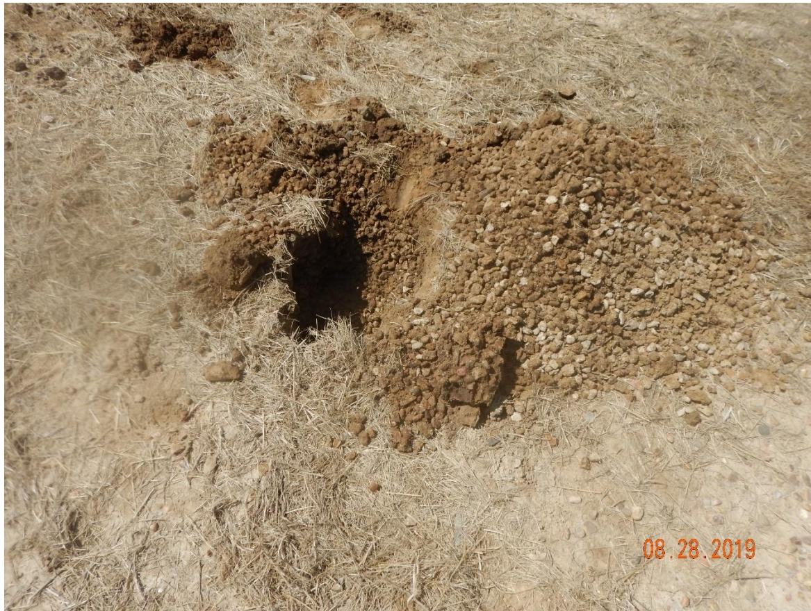
Photo 9: Photo shows gravel material with a chemical smell that was excavated from the test pit.
