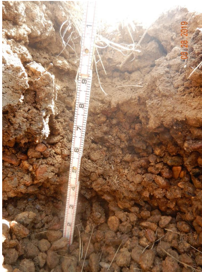
Photo 8: Continued from photo 7. Photo shows quantities of gravel ~4 inches subsurface. A liquid sheen and a chemical smell was also noticed in the gravel.
