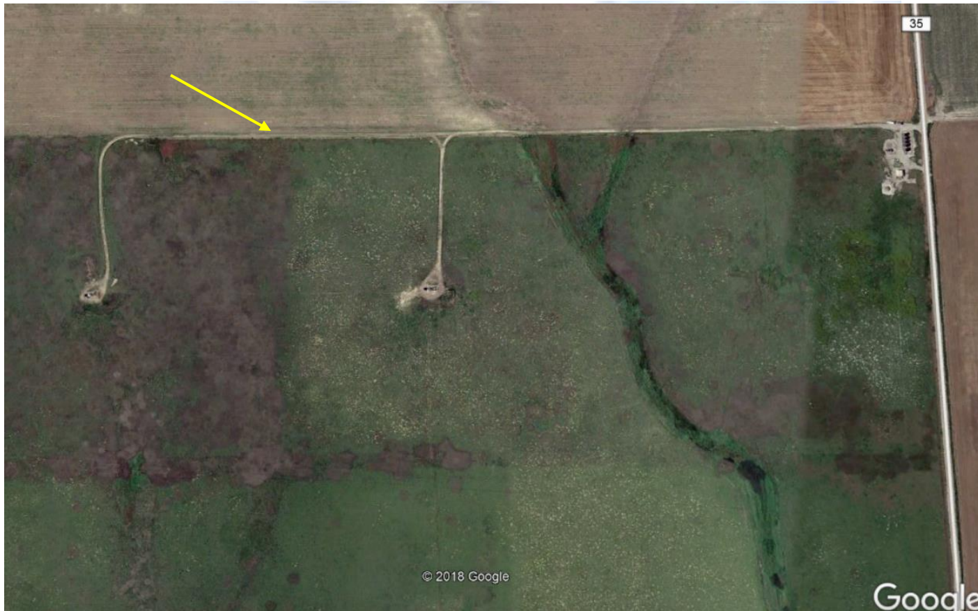
Photo 16: Current available Google Earth aerial imagery (2016). Photo shows Sundance Energy's well locations, battery facility and access roads. Operator has not conducted reclamation on the east/west section of access road (yellow arrow) in accordance with COGCC 1004 rules.
