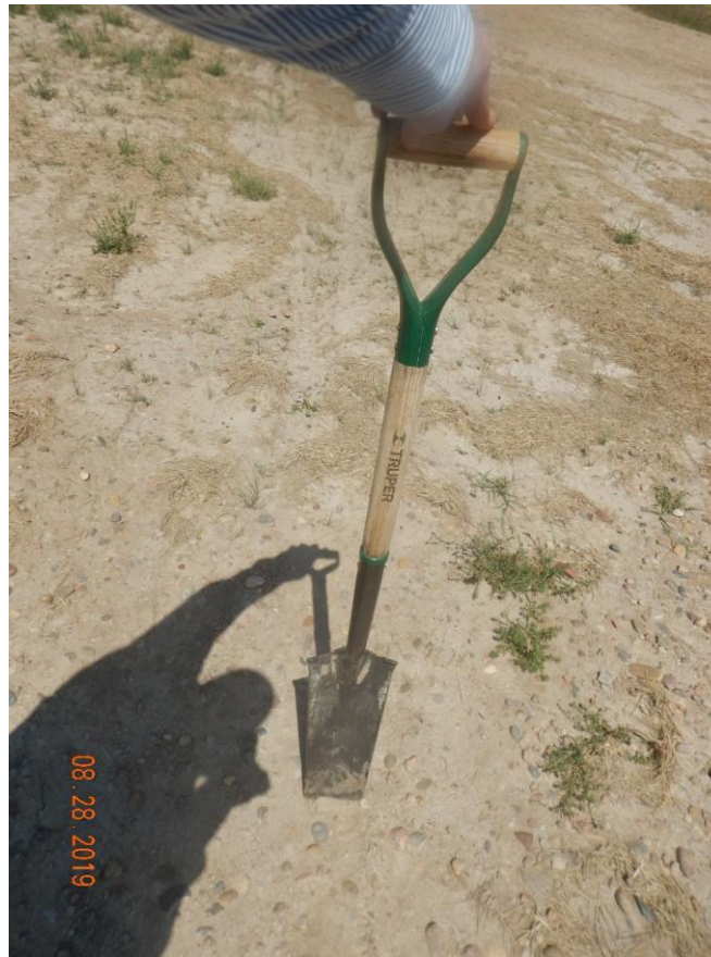
Photo 28: Photo taken from the facility location. Photo shows reclamation specialist tested the location for compaction concerns. Photo shows reclamation specialist was only able to penetrate the top few inches of soil with east. Compaction concerns appear evident
