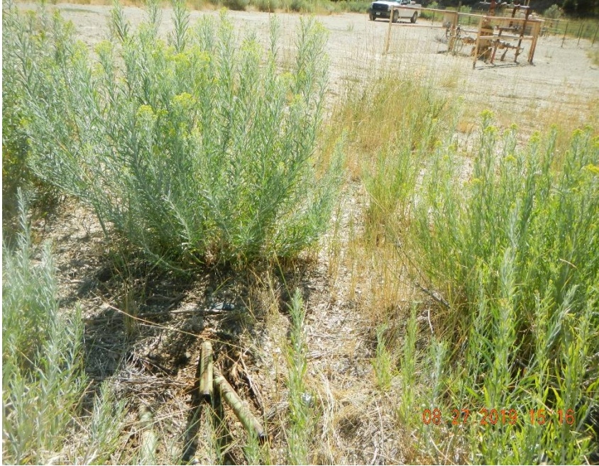
3 unused 1" risers at edge of location between well and tank battery.
