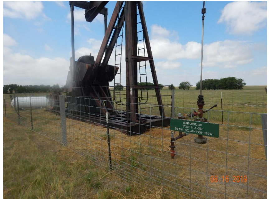
Photo 18: Inspection #696101187 documented weed encroachment at equipment on location and required operator to remove, manage and control weeds. Photo shows vegetation around well appears to have recently mowed, however, vegetation has not been removed from area of equipment. Vegetative growth and accumulation around equipment/wellhead is considered a fire hazard.
