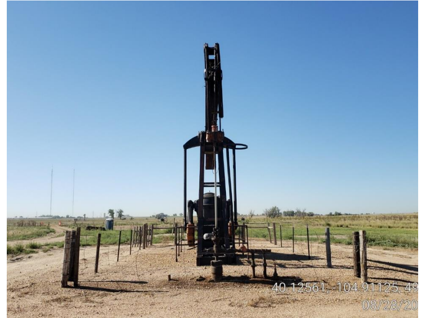
Photo #2 Wellhead & Pump jack
