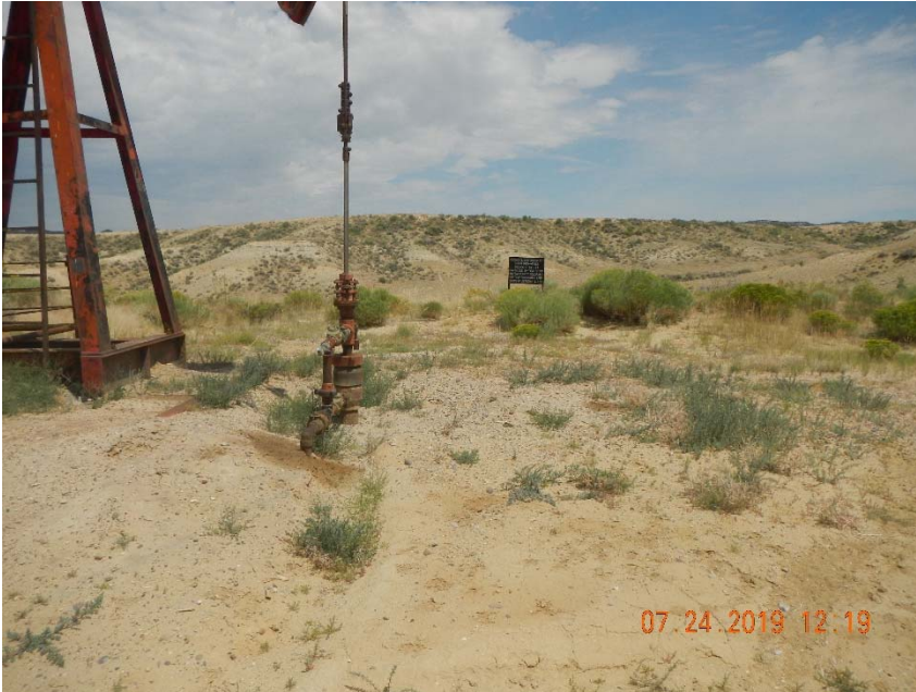
Photo 3. Non-reportable spill – stained soil at wellhead.
