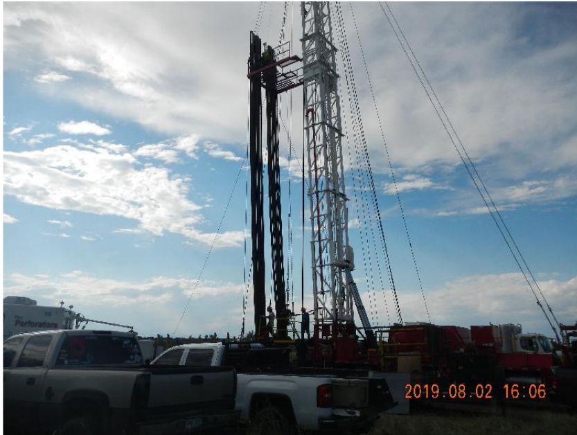
Photo 5: Rig with tubing stands in the derrick.
