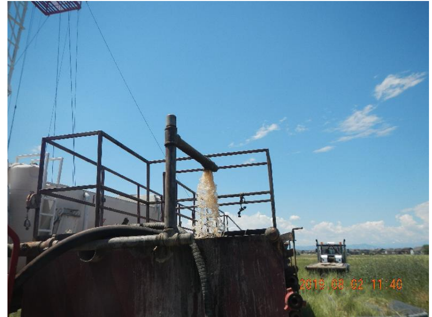
Photo 2: Returns while circulating well.
